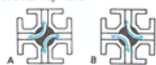
Positions of Four-way Valve
